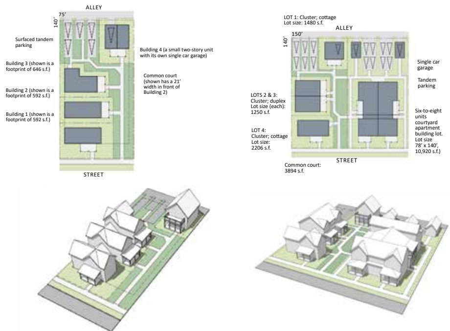
Building form diagrams graphically explain lot frontages, setbacks, height requirements, and other standards for each lot type. Standards are accompanied by photos of local examples to ground the concepts in the local context with familiar sites.
