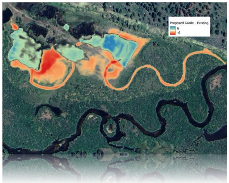
Grading Diagram of Chapman Reservoir Wetlands, RiverRestoration 2026
