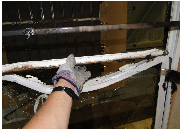
Figure 7.1. This window frame was exposed to radiant heat. The metal-reinforced member (in the back) did not deform when exposed during the exposure interval. The member without the metal reinforcement deflected downward, allowing insulated glass unit to fall out (without initial glass breakage), exposing the interior of the home. Photo: IBHS.
